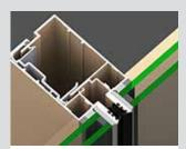
200mm long extruded aluminium retention brackets at mid span and 200mm up from the bottom reduces the risk of mullions seperating.
